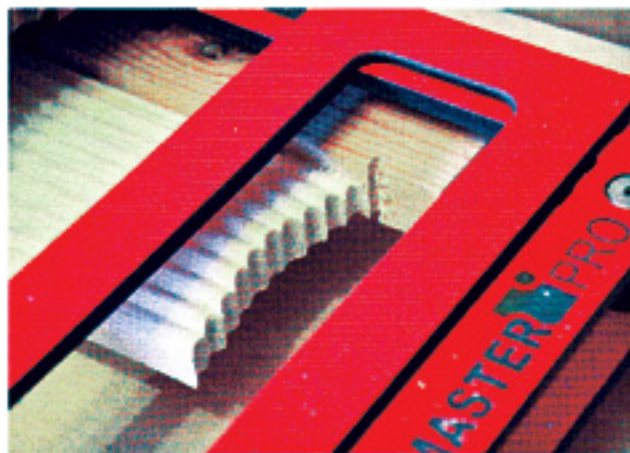
▲ The resulting cut is crisp; note the sacrificial block which remains in place and can be used for fast setup on subsequent cuts
