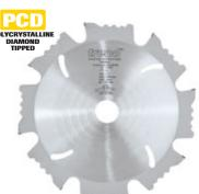
Polycrystalline Diamond Tipped for use in circular saws to rough cut Gemstone worktop. Eight high quality industrial PCD tips for roughing cut leaving 5mm overhang for router trimming. Blade can also be used on cement bonded board.
