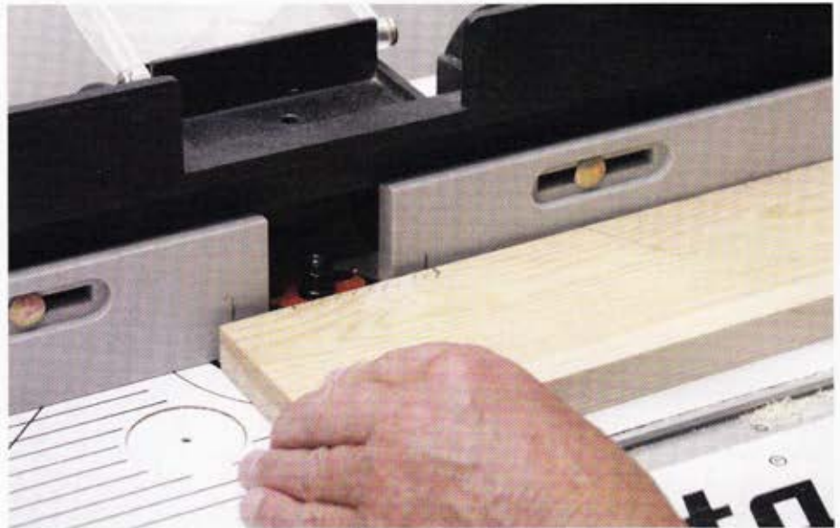
7 Pivoting the board into the cutter. Note pencil marks on fence. The guard is raised here for photographic clarity
