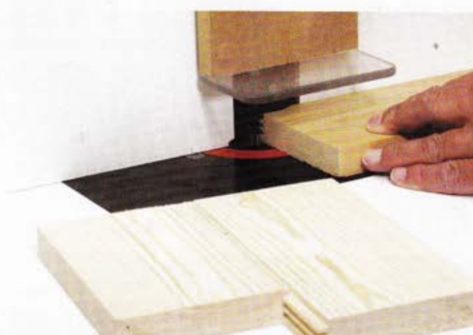
10 The Wealden finger joint cutter, assembled to edge-joint 20mm thick boards
