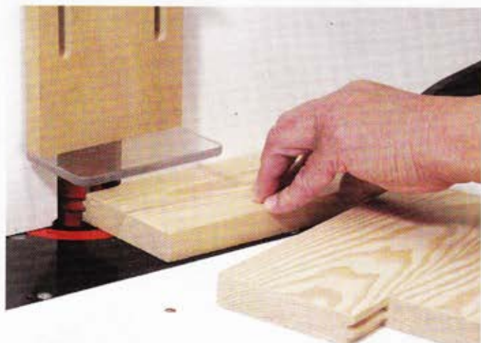
9 Cutting a reverse glue joint. A completed joint can be seen in the foreground
