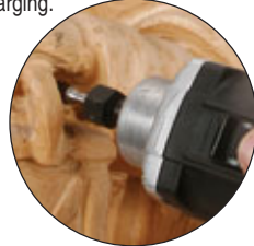
Mini burrs and rasps are ideal for intricate modelling.
