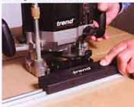
A series of parallel grooves being cut using the CGS attachment
