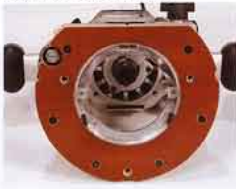
The router base showing the bottom end of the Quick Raiser (upper left)
