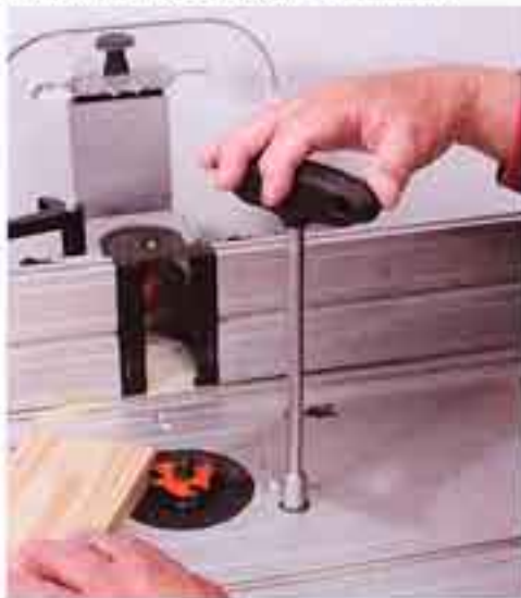
A slotting cutter being set precisely with the T-handle for biscuit jointing in the PRT
