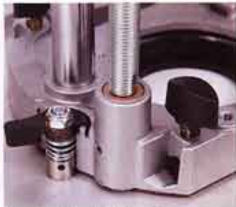
The router in the PRT plate, with one of the quick release levers engaged
