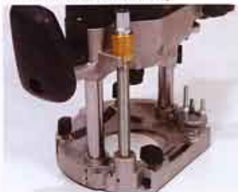
A series of parallel grooves being cut using the CGS attachment
