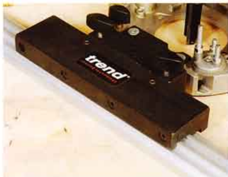
This smart piece of kit screws to the base so that you can slot it onto the Trend Clamp Guides when routing straight cuts such as housings, clearing the work area of clamps so the router passes freely (£37.67)
