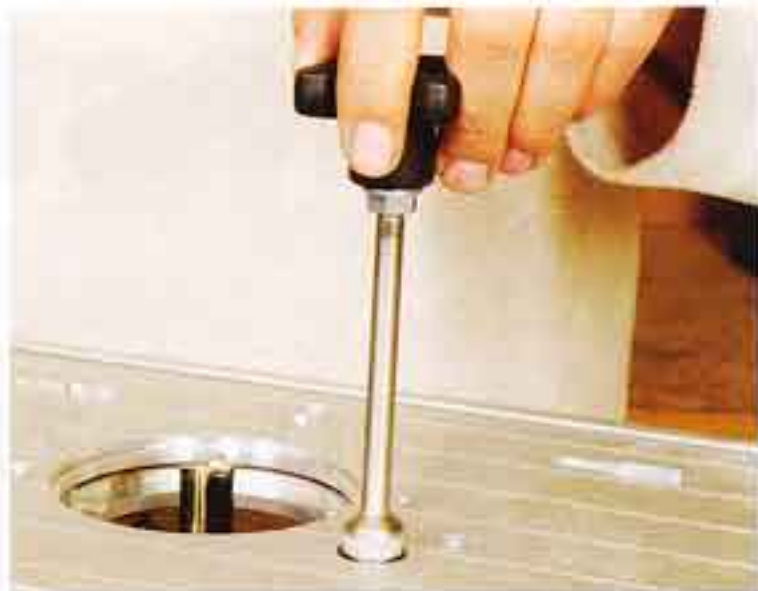
This is where the T11 stands head and shoulders over the opposition, as all height setting is carried out from above the table. Here it is in the Trend PRT table, but any table with a correctly positioned hole drilled through will work
