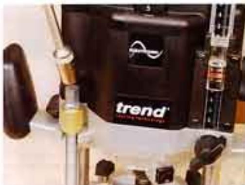
A separate adjuster alters the fine height setting when the router is used in hand held mode
