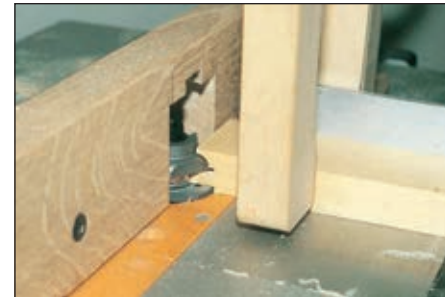
Moulding and grooving a door frame member with the Easyset system
