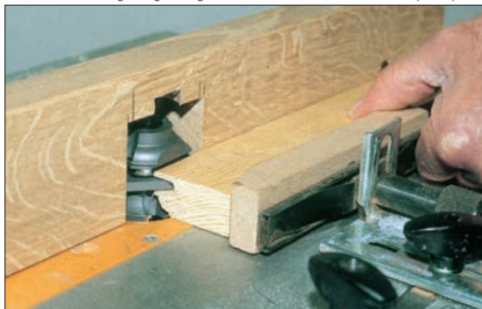
Moulding and grooving a door frame member with the Easyset system
