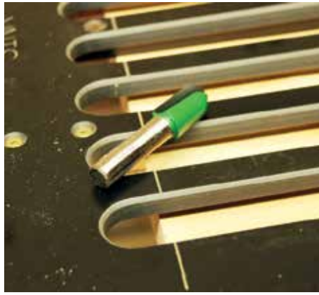
▲ The jig comes supplied with the correct cutter as well as a 30mm guide bush
