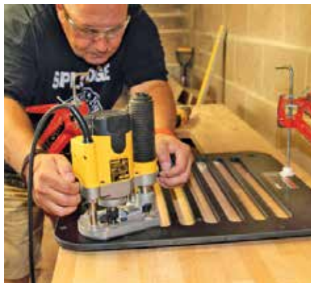
▲ Make each pass through the jig until they are all routed
