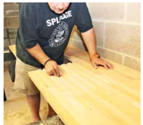
▲ A bit of light sanding and it's ready for fitting and finishing
