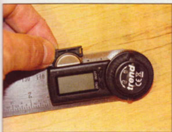
The tiny 3V lithium battery has a 200-hour life and is easy to replace
