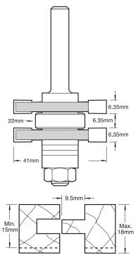
Tongue & groove joint showing minimum and maximum possible timber thickness.
