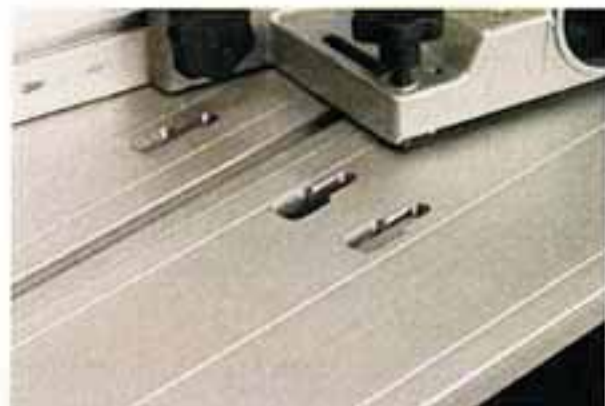
The fence housing locks onto the table with tee bolts in slots.
