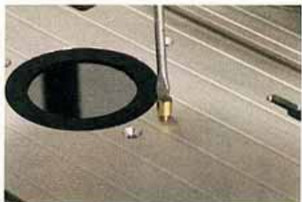
The lead-in pin locates forward of the cutter.
