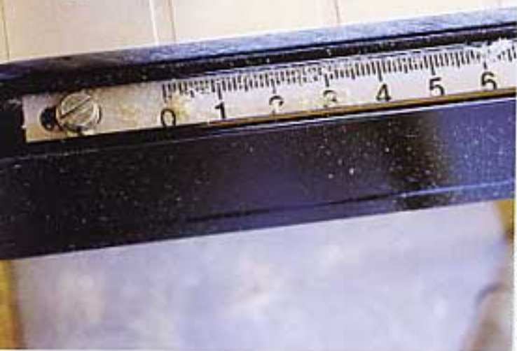
The measuring scales are fully adjustable
