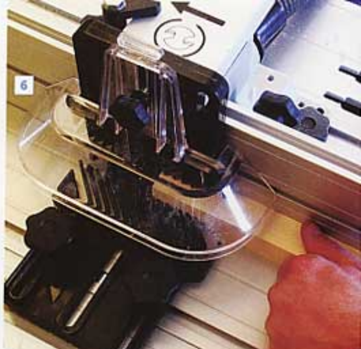
Profiling using the pressure fingers
