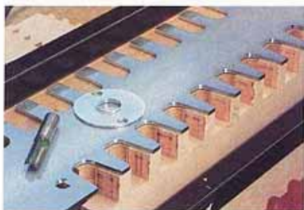
For through dovetails, cut each part of the joint separately: pins are cut with a straight cutter using one side of the comb...
