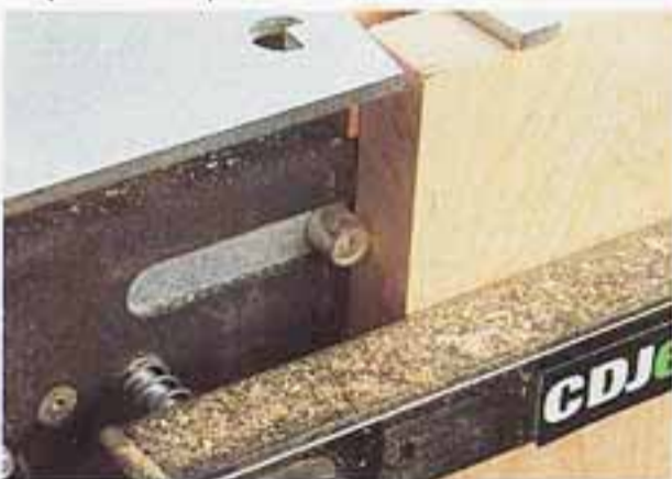
Spring-loaded adjustable clamps hold the work in place.
