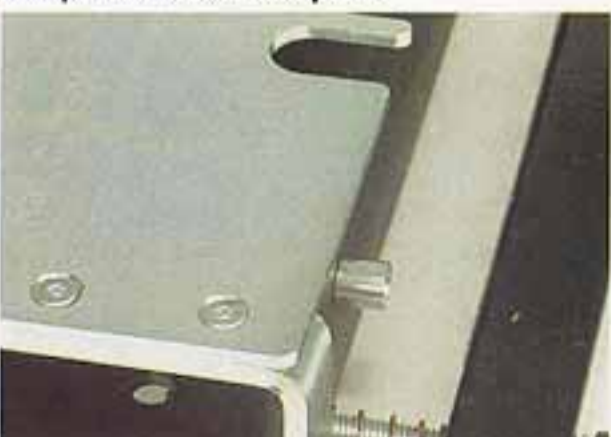
Spring-loaded adjustable clamps hold the work in place.
