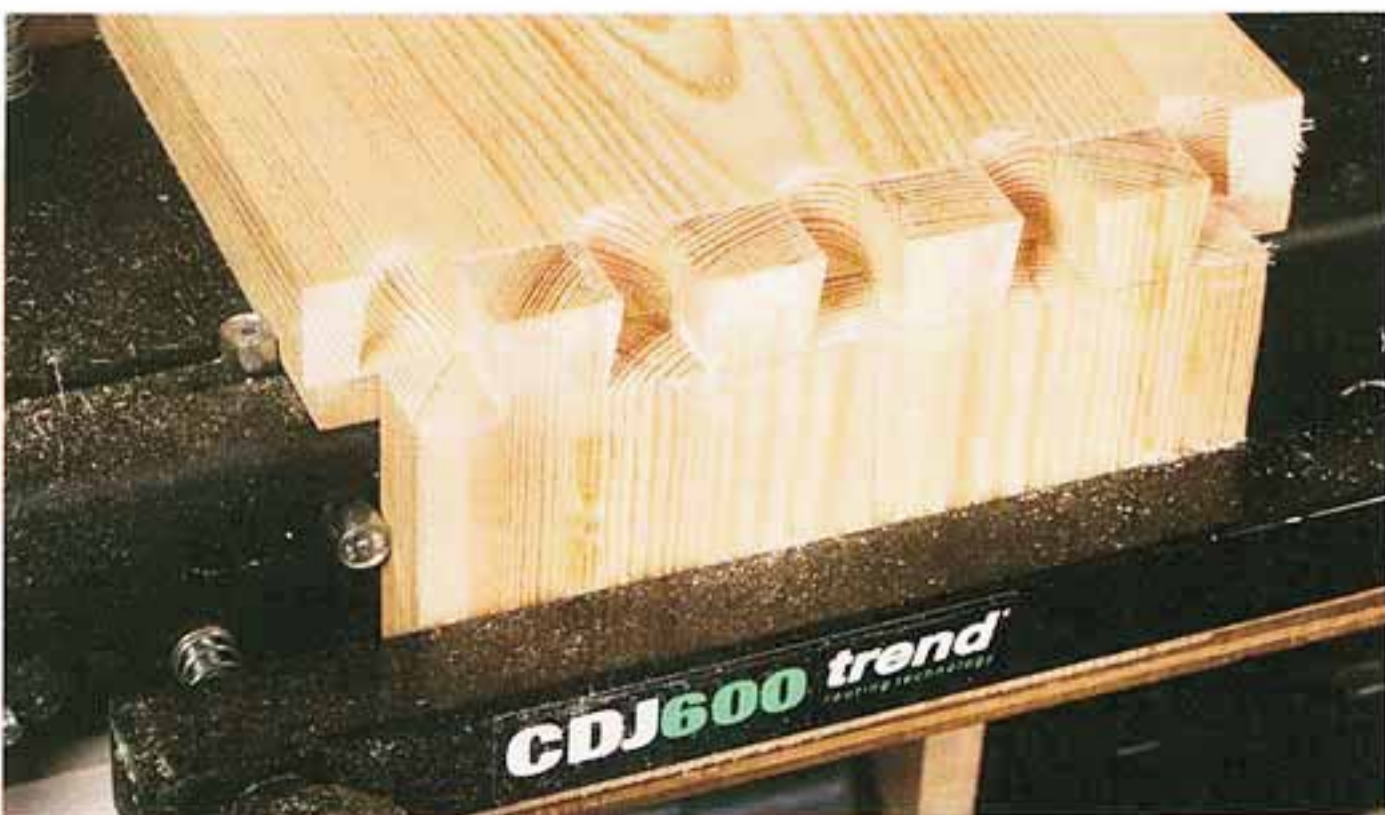
Completed cut. Top board is inserted to prevent breakout.
