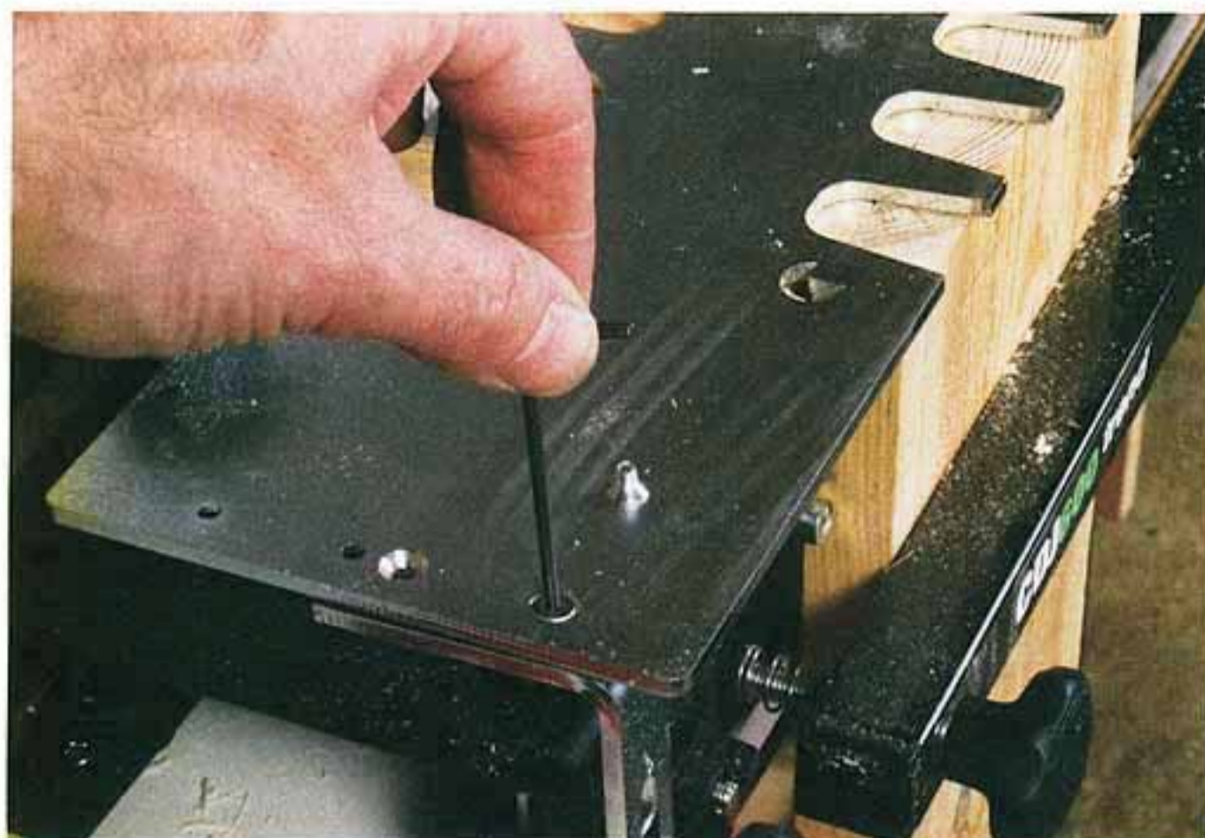
Re-fitting template to cut pins
