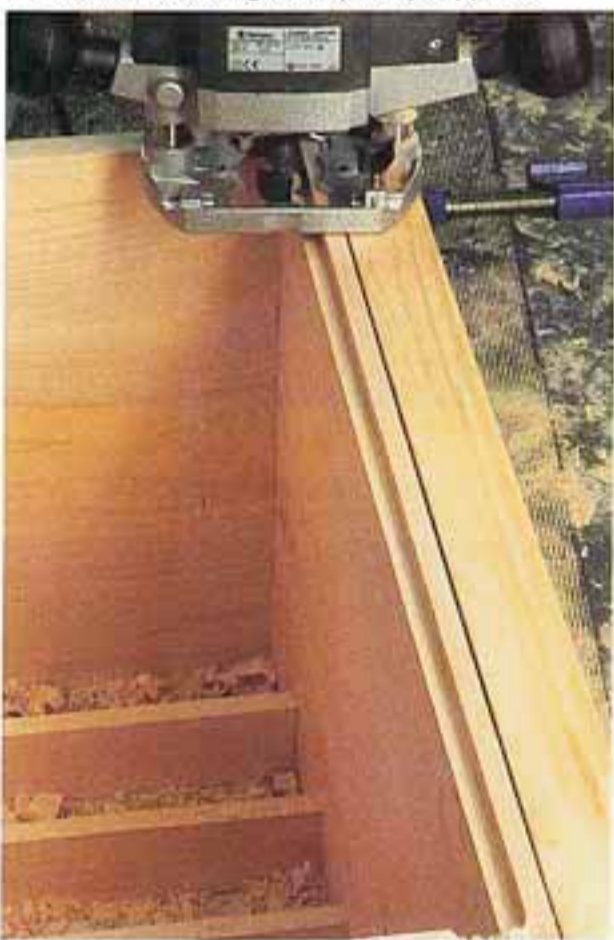
29 Run a rebate around the back of the cabinet using a temporary support.
