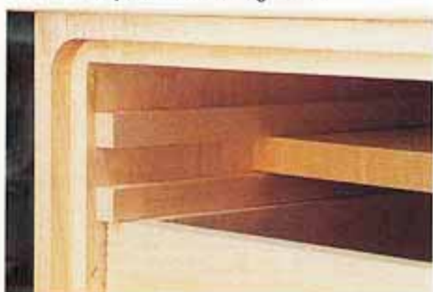
41 Use the two drawer runners on top of the slide to guide it.
