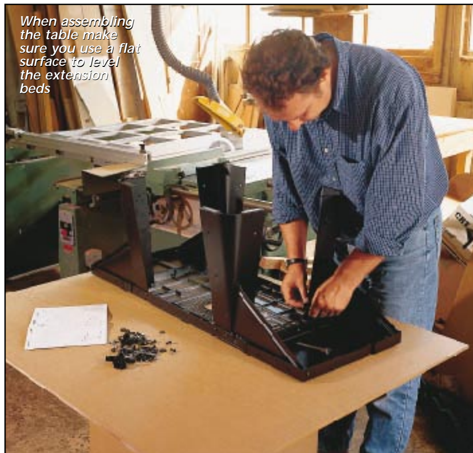
Fit the first part of the Plungebars to the baseplate...
