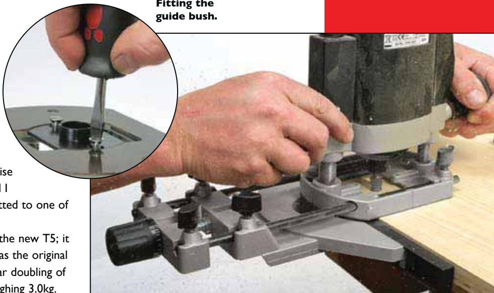
Micro adjustment side-fence.
