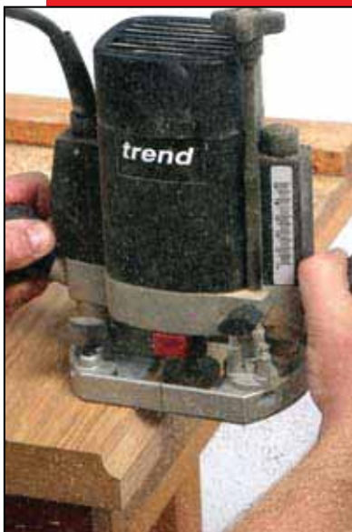
...and with a bearing guided cove cutter Ref. 46/264X1/4TC.
