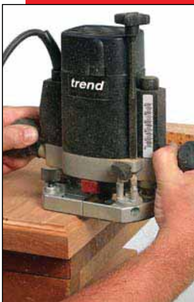
Edge profiling with a bearing guided ogee cutter Ref. 46/30X1/4TC.
