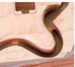
Small wooden tabs hold the guitar to the blank.
