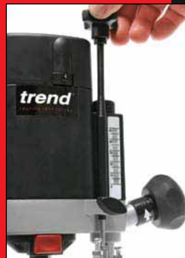
Adjusting the fine height adjuster.
