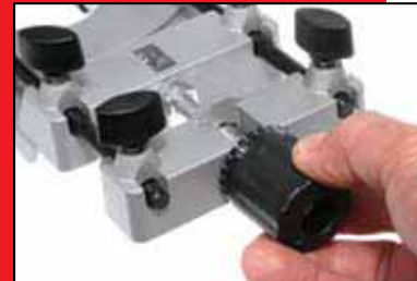
Adjusting the fence using the microfence adjuster.
