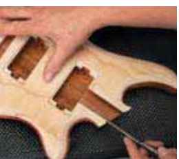
Making adjustments to the neck aperture.
