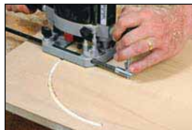
Using the beam trammel bar to make circles and arcs.
