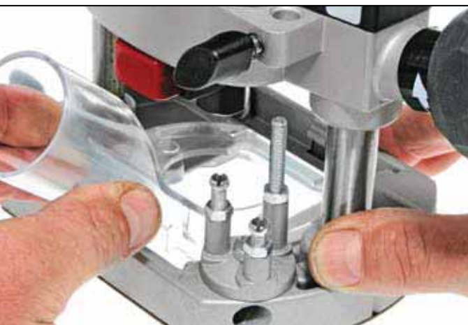
Fitting the new low profile dust spout.
