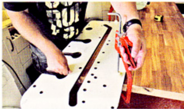
▲ Push the jig so the pins sit tight against the work and then clamp it well
