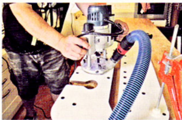
▲ Use the pins to set the jig for the connector bolts
