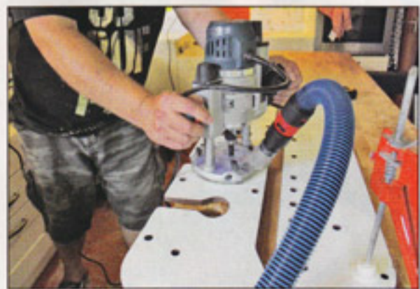
Use the index pins again to position the jig for routing out the connector bolt holes
