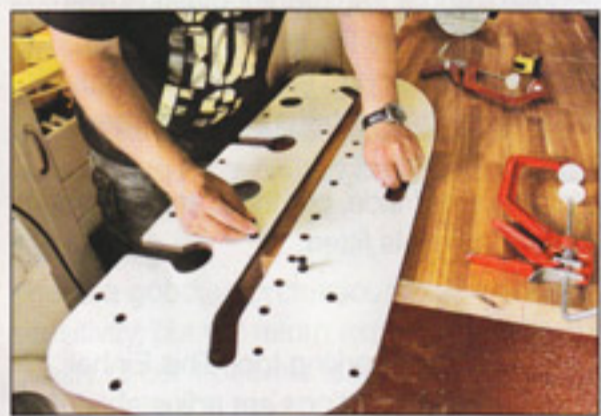
Insert the index pins to suit the cut you're making; then clamp the jig to the worktop
