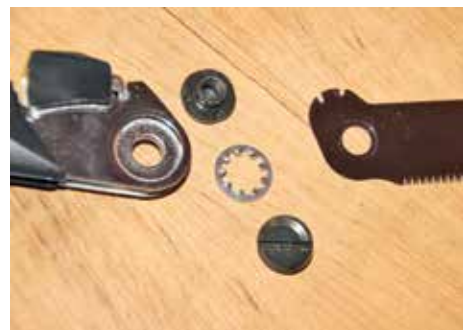
▲ The saw strips down for blade replacement as needed
