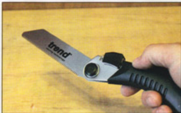
...or cranked back so the handle is held away from the cutting line
