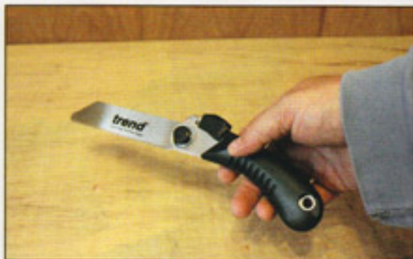
You can use the saw with the blade in the conventional straight position...
