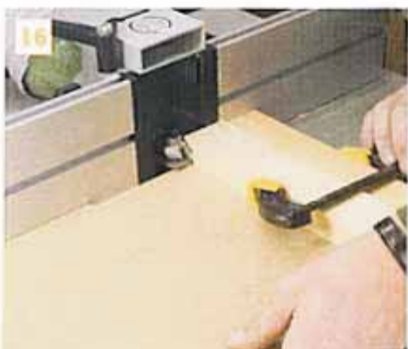
Push the whole assembly through the cutter in a smooth action
