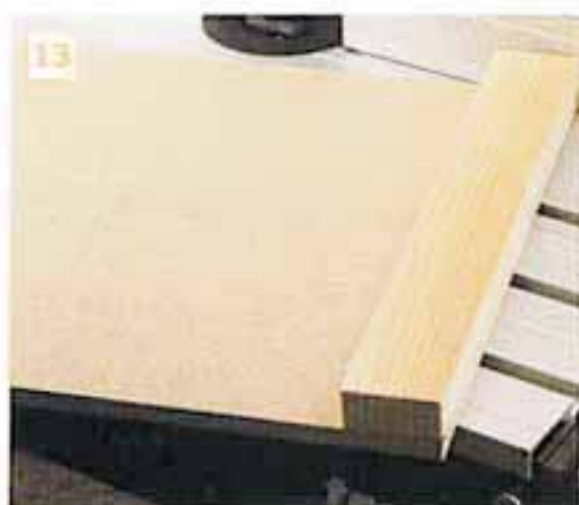
The only critical requirement is that this stop is at a perfect 90° to the edge of the MDF
