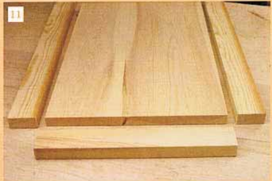
The length of the rails need to be calculated to allow for the stub tenon
