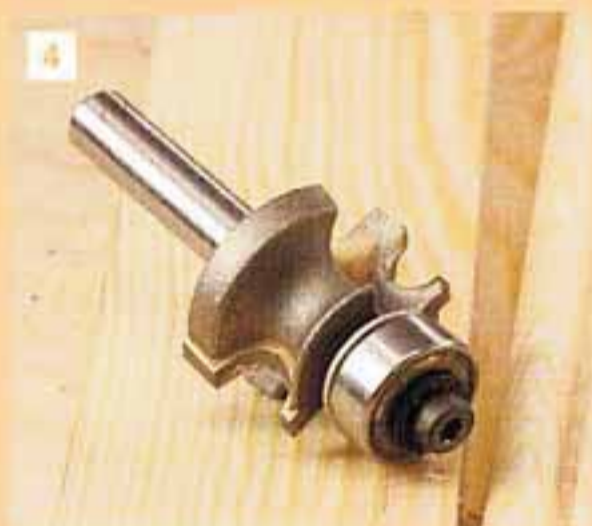
4 Use a bead cutter to form a false groove
