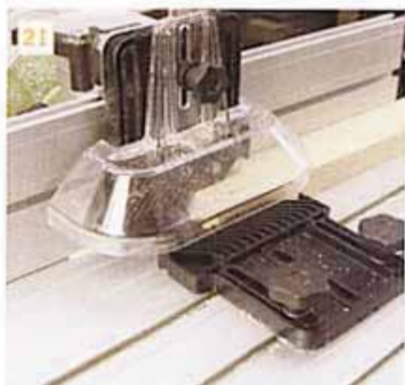
Run the mould down the edges of each of the stiles and the rails
