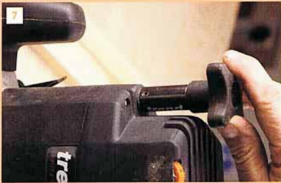
It is essential that your router is fitted with a fine height adjuster
