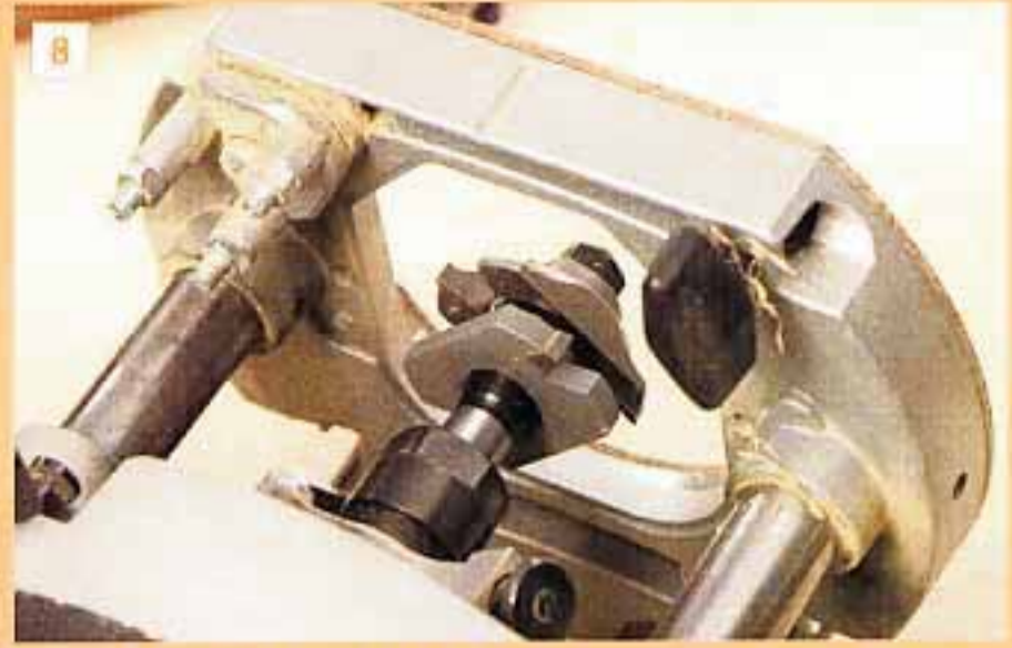
Ensure that at least three-quarters of the shank is gripped in the collet
