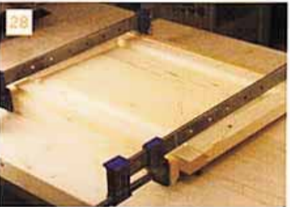
28 Glue the frame joints and clamp the whole thing together
