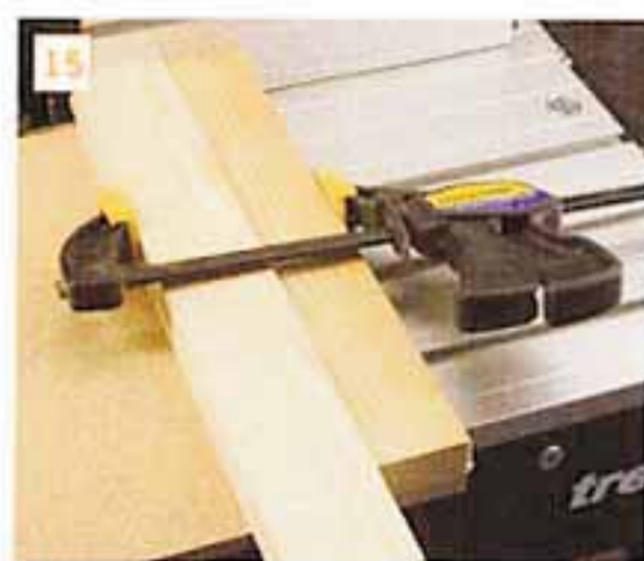
Clamp the rail to the guide jig, making sure both of them are tight against the fence
