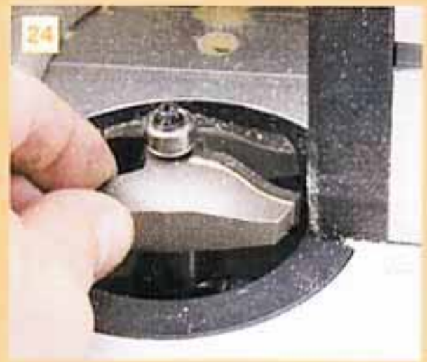
24 Revolve the cutter by hand to make sure there really is enough clearance
