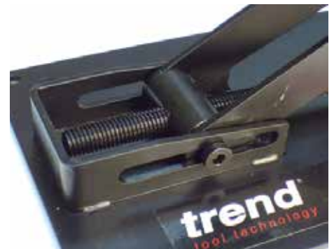
The steel pin joints are robust, operate smoothly and shouldn't need lubrication, though you'll obviously need to clean out sawdust if it accumulates
