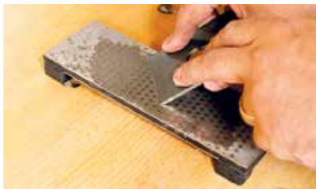
▲ Used with the bench stone the rubber construction keeps everything secure to the bench
