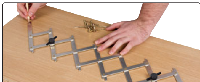
Simply expand the point to point mechanism, find the ideal spacings and lock the 7-point marking positions, then transfer to component.
