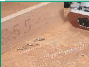
Both numeral and alphabet templates can be used with alternative cutters to produce rounded, moulded or Vee cut lines, all using the same diameter (13mm) guide bush.
