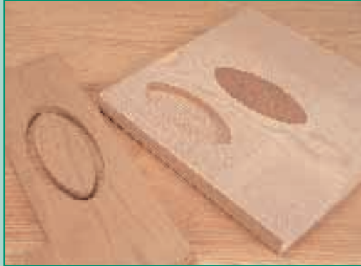
The timber repair template can also be used for inlaying contrasting timbers, veneers or laminates
