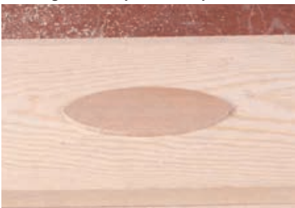
Patch glued and pressed in place
