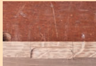
Hinge recess routed with familiar rounded corners
