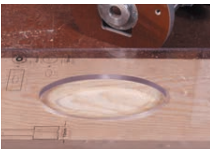
Patch glued and pressed in place
