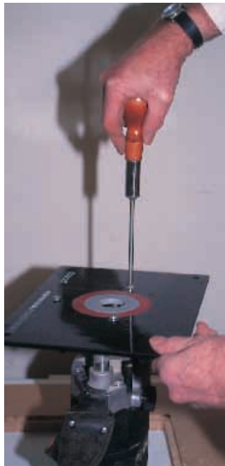
Fixing the router to the insert
