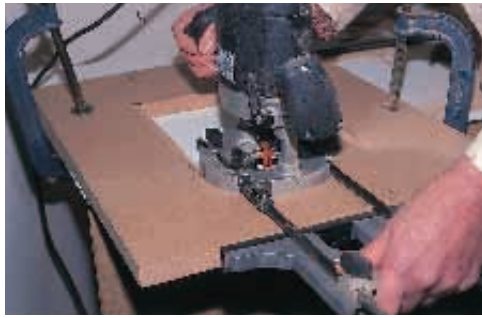
Forming rebate using straight cutter
