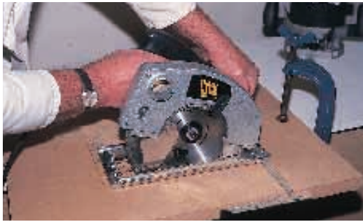
Alternative method of removing waste with a circular saw
