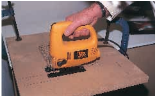
Even when using the circular saw, a jigsaw completes cutting in the corners
