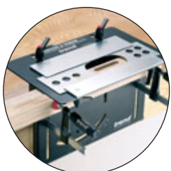
Routing the mortise
