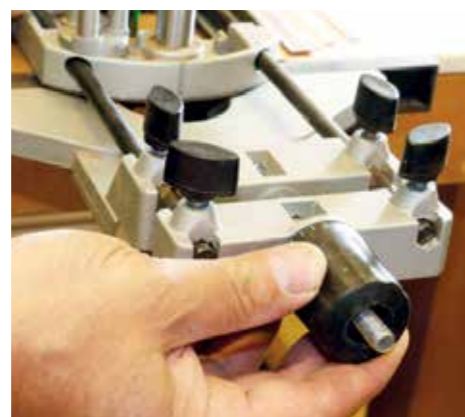
The fence is excellent and comes with a fine adjuster as standard
