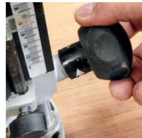
The simple twist lock plunge is great for fast, easy and controllable plunges
