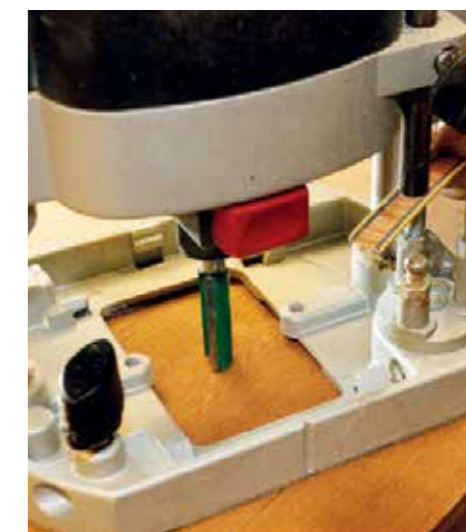
... or against inlays to set the routing depth to let them in perfectly flush
