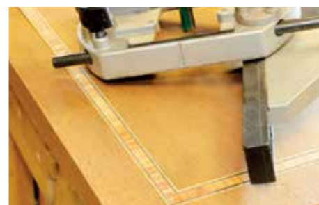
The basic T5 is very adaptable and not just limited to edge moulds; this inlay is easy to let in but very effective
