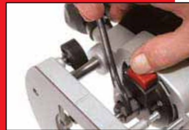
Using the spindle lock to tighten the collet nut.
