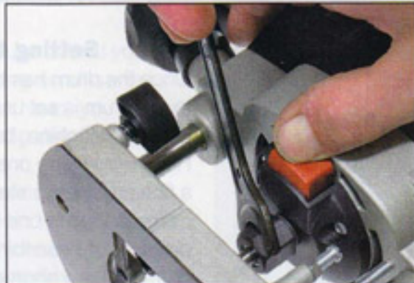
The spindle lock makes it easy to change cutters
