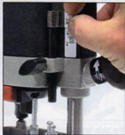
The depth stop is the ubiquitous rod type
