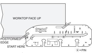
Release plunge on router at end of each cut.
