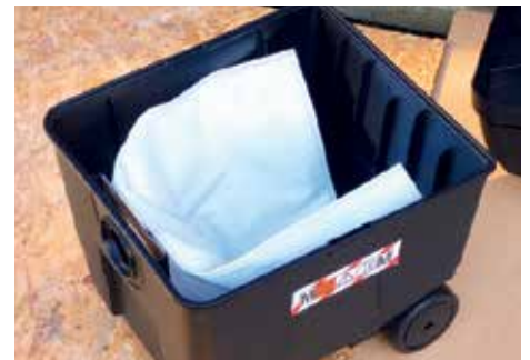
Inside the plastic drum is a disposable fabric collection bag, slotting into a groove just inside the inlet
