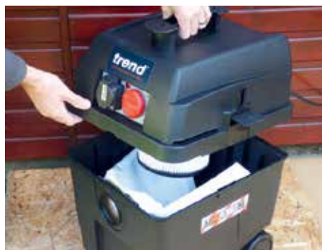
The lid contains a powerful 1,400W motor and is detached by flipping open a couple of locking levers
