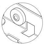
Make sure guide bush collar is fitted with chamfered edge facing the jig when parked. This will make it easier to remove.
