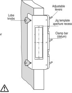
The jig template aperture recess notches in the jig central aperture are to be used as an initial visual guide only, always check the jig and template is centred to the door using a rule or tape measure before routing.
