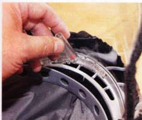
▲ Pic.1 This little device measures airflow to indicate if the filters need changing
