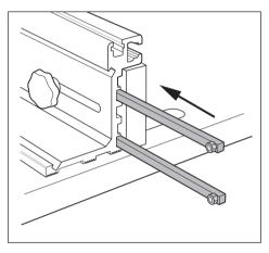
The rods can be parked in the T-slots in the top of the back fence. The rods are held by tightening the knobs.
