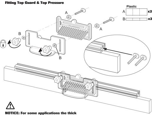
NOTICE: For some applications the thick and thin washer can be swapped over. For example, when profile scribing using a pushblock.
