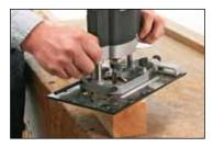
**Multiple grooving.** To repeat a series of evenly spaced grooves the CRB is drilled to take a small copy batten which you machine up to be a sliding fit in the required groove. Make the first cut using a straight edge or clamp guide, screw the batten onto the CRB, then locate this in the first groove and make a
