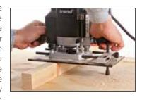
using fiddly ski supports. You can use it on work between 8 and 80mm thick. My criticism here is that the end of the leg has some form of soft plastic knob which tends to drag on the support surface. It needs to have a highly polished hard surface for a smoother movement, otherwise it is dead easy to use and very useful.
