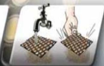
Mesh can be easily cleaned. Just tap out the dust or rinse, dry and re-use
