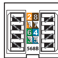
Fig. 2 568B Terminals Colour Coding
