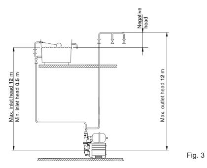
Before deciding where to locate the unit, check to ensure the static inlet head (Fig. 3) meets the minimum requirement of 0.5 metres and does not exceed the maximum requirement of 12 metres.
