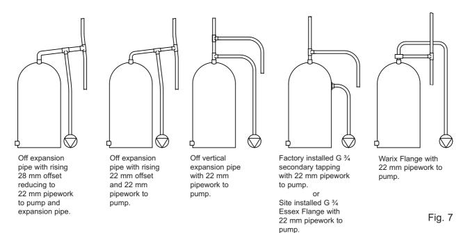
Pipework Connections (Connection between pump and system outlet)
