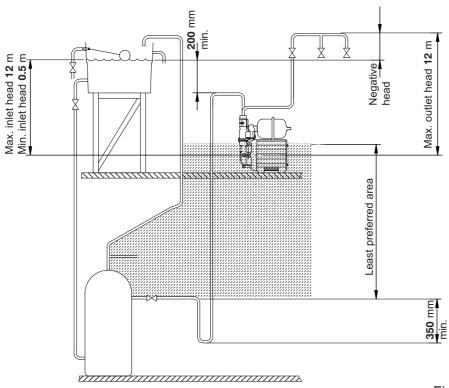
Note: Ensure water surface is a minimum of 200 mm above highest point of inlet pipework at all times to prevent air locks.
