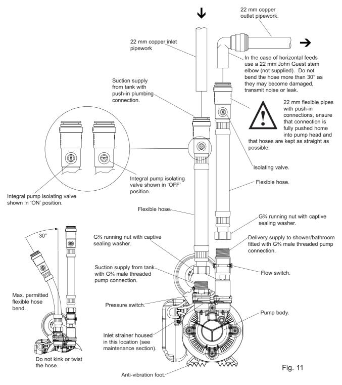
The pump should not be screwed down, ensure anti-vibration feet and flex hoses are used.
