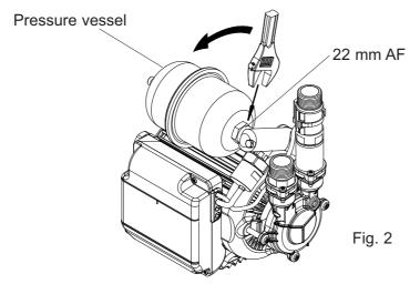
The pressure vessel (Fig. 2) is factory fitted to the pump assembly.
