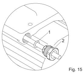
To enable correct assembly of the cable gland the 'O'-ring (Fig. 15 item 1) must be placed over the cable before the clamping insert (Fig. 15 item 2) can be tightened. Note: Cable diameter range:- 6.5 mm to 9.5 mm.
