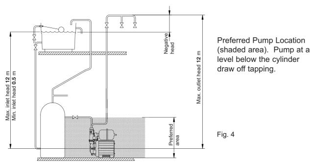
Before deciding where to locate the unit, check to ensure the static inlet head (Fig. 4) meets the minimum requirement of 0.5 metres and does not exceed the maximum requirement of 12 metres.
