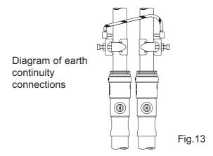
Certain installations may require additional earthing arrangements such as equipotential bonding. Reference should be made to the relevant regulations concerning this subject to ensure compliance.
