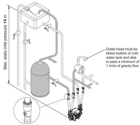
Positive Duty Twin Pump System Fig. 5
