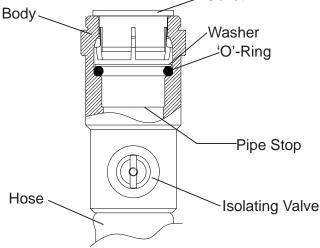
4. Push pipe firmly into fitting, until pencil mark is level with the top of the collet and the pipe stop resistance is felt. Pull on pipe to check it is secure and correctly fitted.
