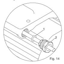
To enable correct assembly of the cable gland the 'O'-ring (Fig. 14 item 1) must be placed over the cable before the clamping insert (Fig. 14 item 2) can be tightened.
