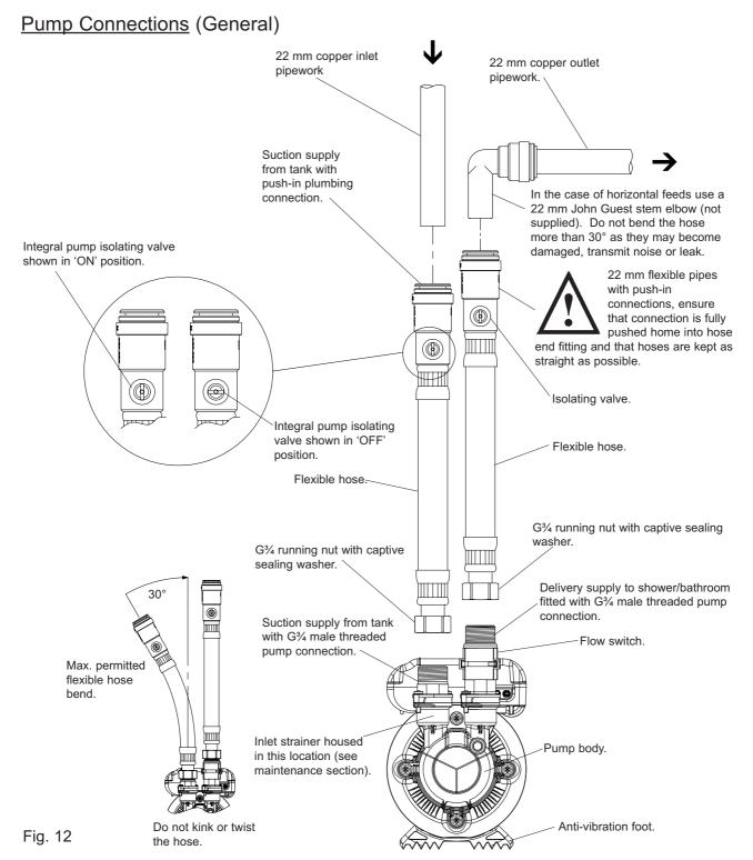
The pump should not be screwed down, ensure anti-vibration feet and flexible hoses are used.
