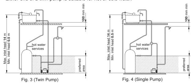
Preferred Pump Location (shaded area). Pump at a level below draw off tapping in cylinder.
