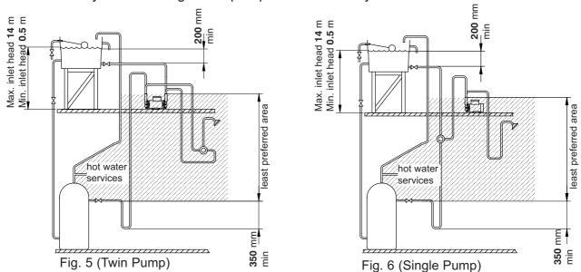
Least Preferred Pump Location (shaded area). Pump located above the hot cylinder can increase the risk of air locks.
