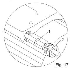
To enable correct assembly of the cable gland the 'O'-ring (Fig. 17 item 1) must be placed over the cable before the clamping insert (Fig. 17 item 2) can be tightened. Note: Cable diameter range:- 6.5 mm to 9.5 mm.
