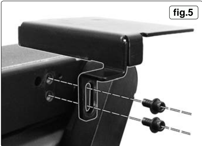
4.4 Attaching the sanding belt work support/guard. 4.4.1 Referring to fig.5 above, position the slotted mounting leg of the work support/guard over the two threaded holes in the side of the belt housing and fix in place using the two socket cap screws and washers provided. Screw them down, finger tight only at this stage. Supporting the underside of the work support/guard, lift it slightly so that there is at least 1.5mm of clearance between the support and the surface of the belt and then fully tighten the bolts using a 6mm hex key.
