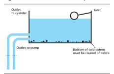
In systems with more than two bathrooms, the cold water supply to the cylinder must be in 28mm pipework.
