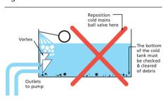
Chronic aeration of the pump occurs when this problem is combined with inadequate storage capacity and/or when the volume of water is drawn by the pump and other services exceeds the refill rate and creates a vortex which draws air and possibly debris into the pump.
