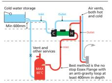
In positive head systems, allow for increased resistance of long pipe runs with multiple bends. The natural flow from the outlets MUST be at least 2 litres/min mixed on hot and cold.
