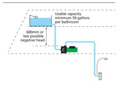
Tank fed, pressurised cylinder or combination boiler system with single-ended Right Universal pump to boost the hot supply water pressure and cold water mains supplies 'cold' to shower, bath, basin and toilet.
