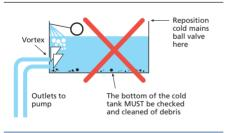
Chronic aeration of the pump occurs when this problem is combined with inadequate storage capacity and/or when the volume of water drawn by the pump and other services exceeds the refill rate and creates a vortex which draws air and possibly debris into the pump.
