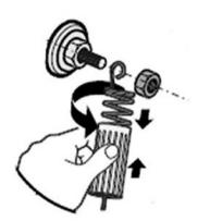
4a. Spring fixings supplied with a sleeve are adjustable. Rotate the sleeve anti-clockwise to shorten and clockwise to lengthen.
