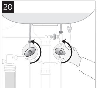
Note: Check all connections to ensure they are tight and that there are no leaks.
