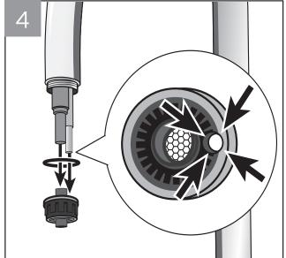
\* NOTICE: Align through hole and push the metal tube all the way through the aerator.
