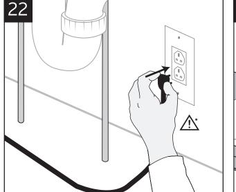
\* NOTICE: Property Damage. Do not use an extension lead with the tap. (A standard earthed outlet within 760 mm (30") of the tap is required under the sink.)
