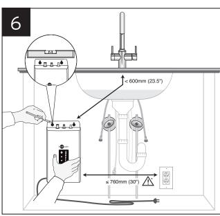
\* NOTICE: Property Damage. Do not plug in hot water tank. Tank must be located within 600 mm (23.5") of tap and within 760 mm (30") or less of a standard earth (grounded) outlet. DO NOT extend plumbing or electrical lines.
