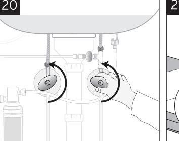
Note: Check all connections to ensure they are tight and that there are no leaks
