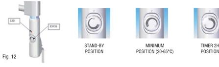
Electrical towel rail must not be installed with the AQUARIUS II regulating box located at the top. This can seriously damage the electronic control box and create a dangerous situation with a risk of fire.
